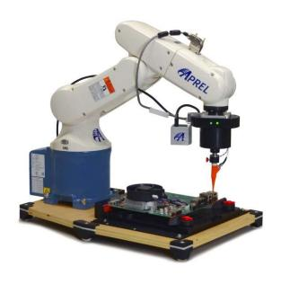
Included in the package is the ability of utilise the EM-ISight vision system which allows for easy DUT setup and ease of reporting. All data captured is aligned with the active scan and vision settings, heat maps can be presented with 2D and 3D overlay based on the real data captured. All data can be exported in raw format for advanced user analysis. Automatically generated frequency plots form part of the software.
